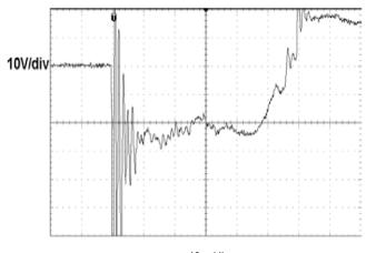
40ns/div ESD clamping voltage Fig 9. (IEC61000-4-2-8KV contact)
