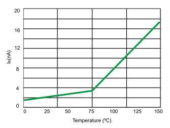
Fig 4. Typical Leakage Current vs. Temperature
