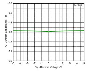
Fig 7. Capacitance vs. Reveres voltage
