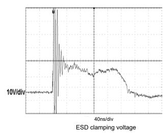
Fig 8. (IEC61000-4-2 +8KV contact)
