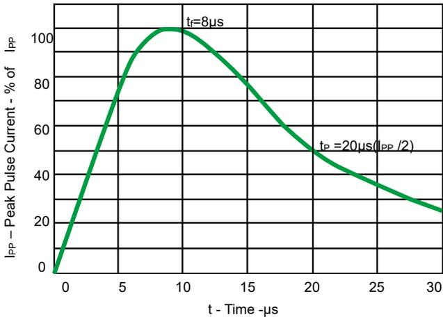
Fig 1. Pulse Waveform
