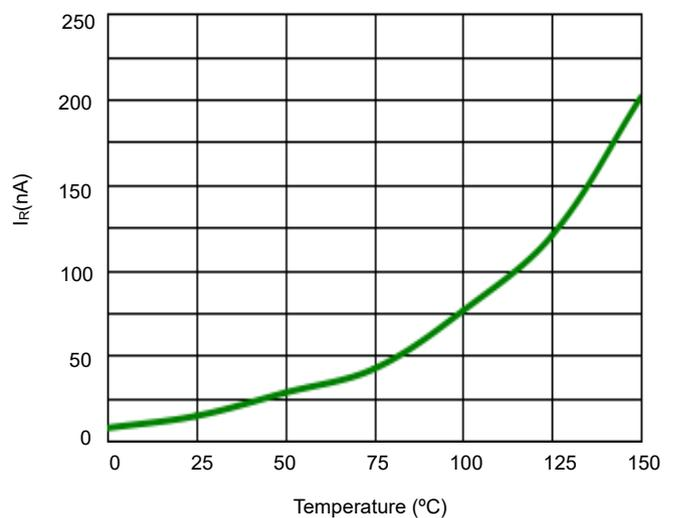
Fig 6. Typical Leakage Current vs. Temperature
