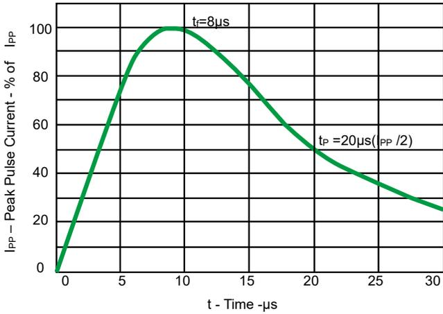
Fig 1. Pulse Waveform
