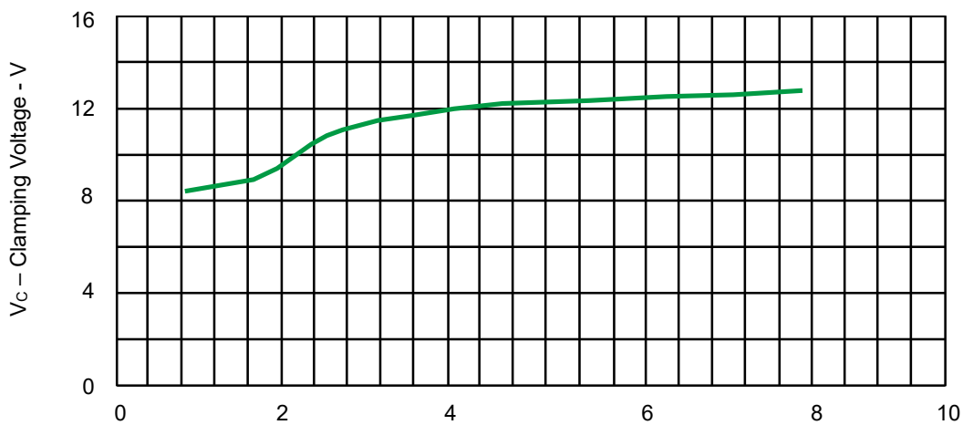
Fig.1 Typical Clamping Voltage VS Peak Pulse Current for PESDNC563T5VU
