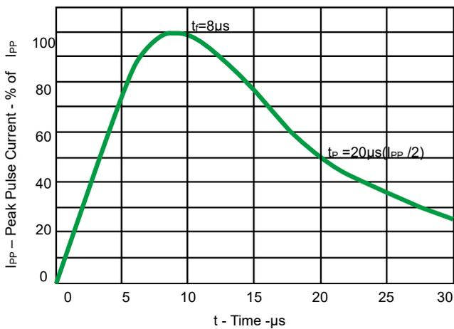
Fig 1.Pulse Waveform
