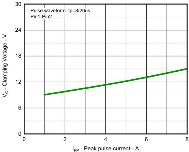
Fig 3. Clamping voltage vs. Peak pulse current
