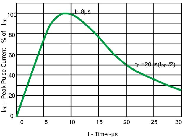
Fig 1.Pulse Waveform
