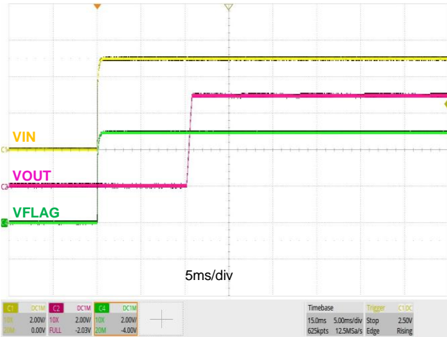
Power on Response( R_{SET}=20k\Omega , No Load)
