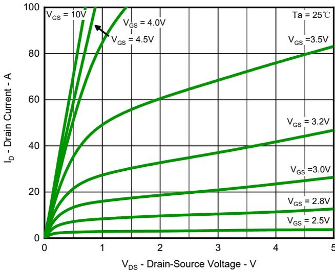
Fig.1 Output Characteristics
